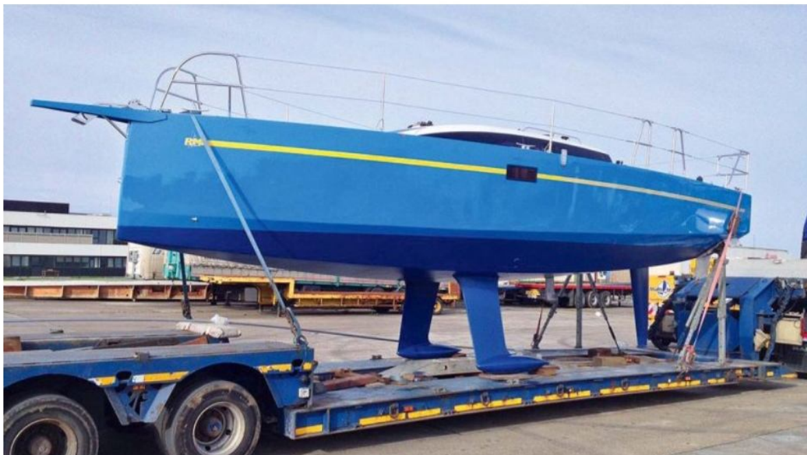
A new RM890 ready to hit the road. The twin keels draw 1.5m. Photo: RM Yachts
