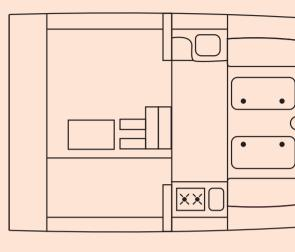
ABOVE: Minimalist and practical interior: no table - instead blue jerrycans form a mezzanine, a tool-box can be used for a seat, elastic strings replace the sliding doors proposed in the original design.
